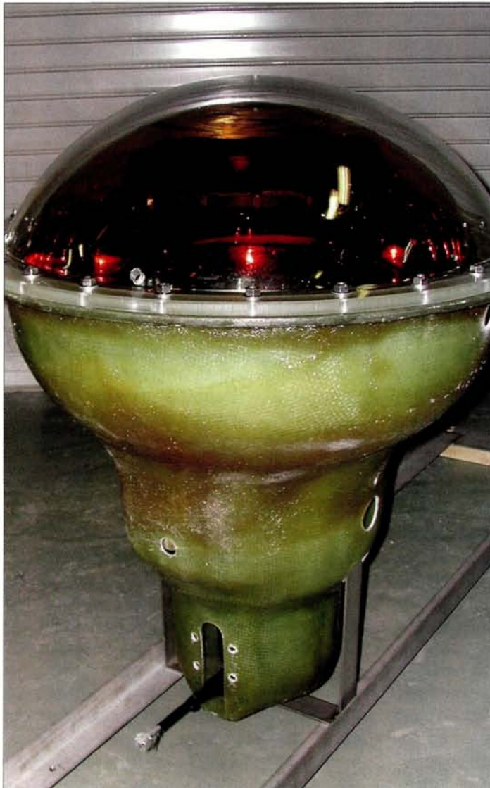
The rebuilt Superkamiokande detector's photomultiplier tubes will be encased in bubbles made of acrylic and fibre-reinforced plastic to prevent shockwave propagation should a tube implode.
